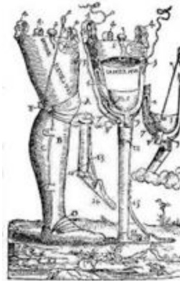
Prosthetic leg designed by Ambroise Pare
